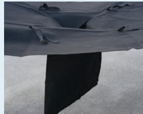
A filter insert, known as a witch's hat.
