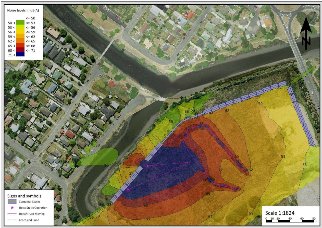
Figure 5.2: Noise contour plot of container yard activities with a gap in the stack of containers along the perimeter.
