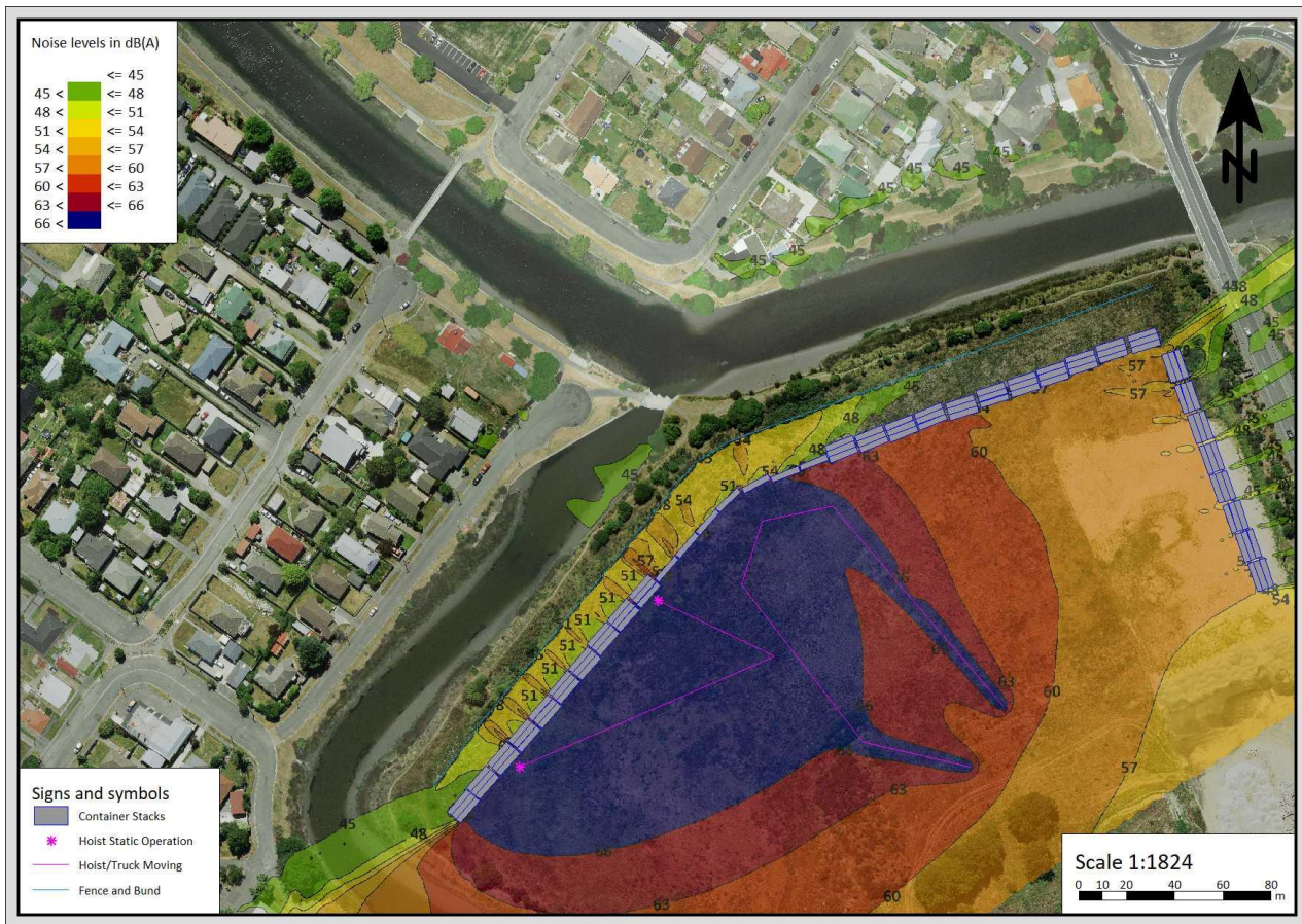
Figure 5.1: Noise contour plot of container yard activities with a continuous stack of containers along the perimeter.
