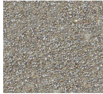
Crusher Dust grit path (Informal footpath)
