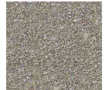
Crusher Dust grit path (Informal footpath)
