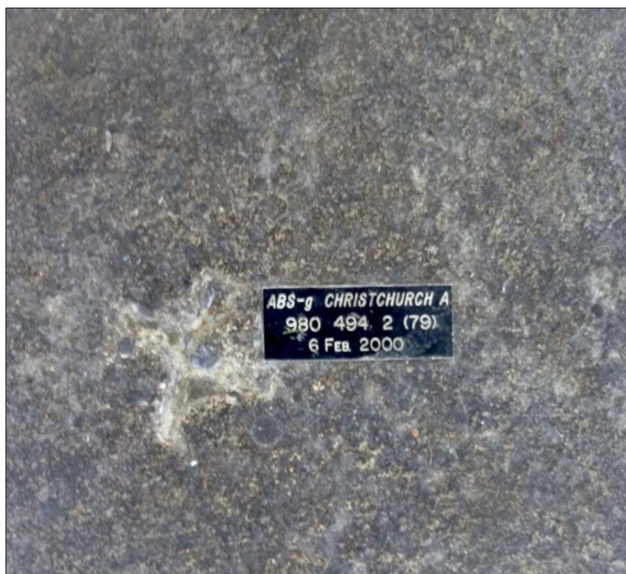
Figure 1.77. The cross in the floor of the Workshop marks the fundamental reference point. The small number plate on the floor was given to the Gardens by the Institute of Geophysical and Nuclear Sciences (GNS) - formally DSIR - to be glued next to the cross.
